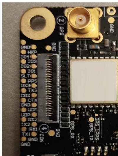
Figure 5 Composite Data Communication Interface
